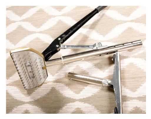
The use of a power stretcher is mandatory. Devices used as a substitute for, or an attachment to, a power stretcher may cause injury, damage carpet, sub-floors, or result in an inadequate amount of stretch and are not acceptable.
