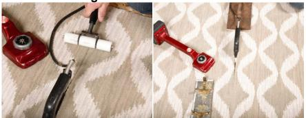
Installers must check with the tool and seaming tape manufacturers for the proper heat settings and tapes. When seaming, we recommend working from the seam midpoint to the seam ends.
