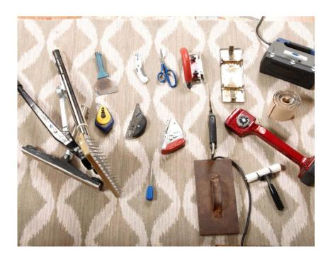
**Examples of some of the tools needed for installing carpet**
